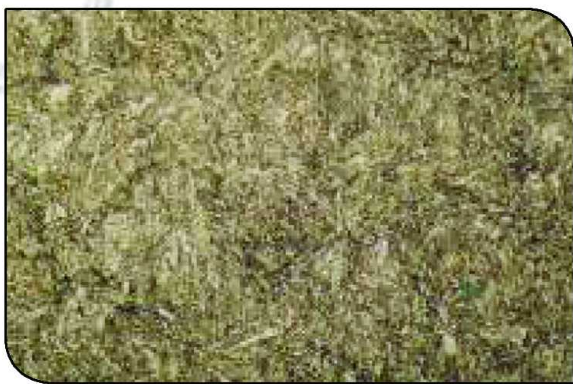
SB H 62F- Tempered martensite(x200)
